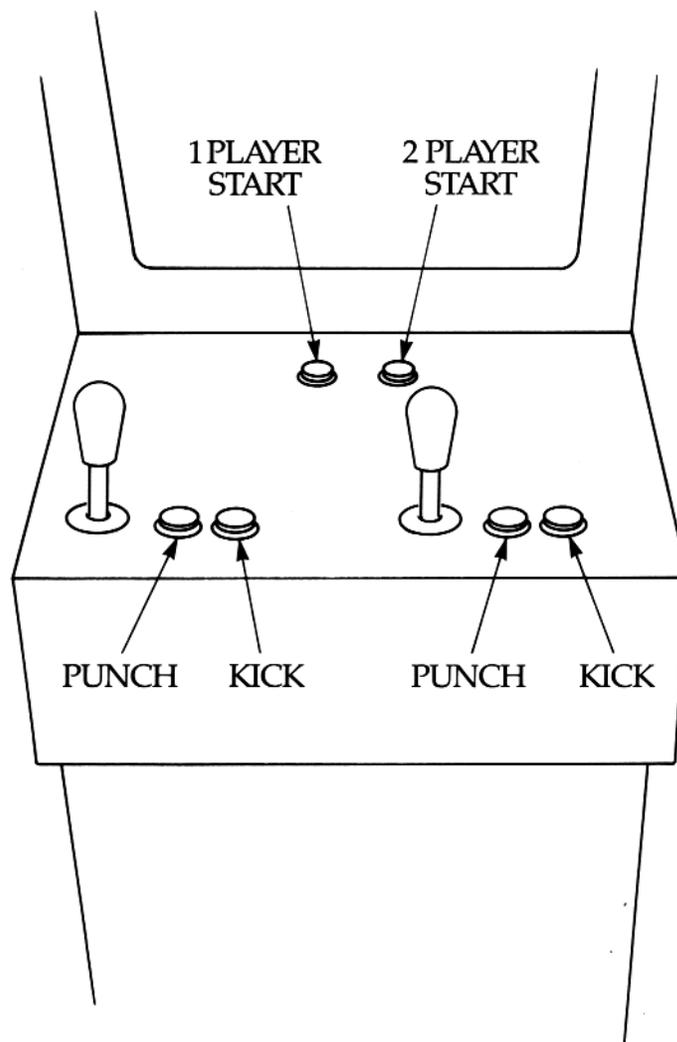
\*When making this 2 player conversion, only the standard JAMMA harness is necessary. Be certain to follow the connecting diagram carefully.
