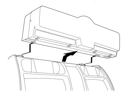
5. Remove the Header Assembly
