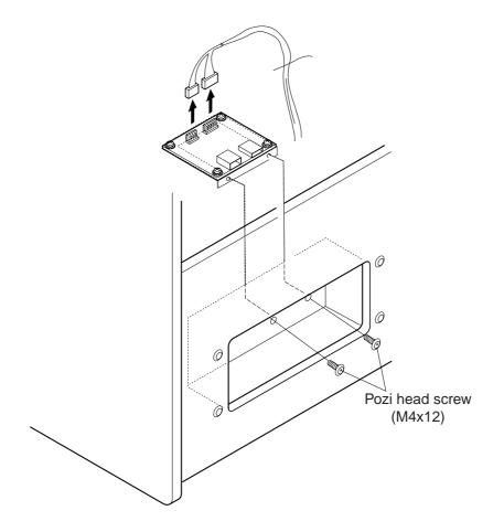
4. Refit the new Link PCB complete with mounting bracket using the 2off pozi head screws (M4x12).
