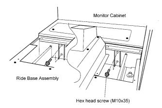
4. Pull the ride assembly away from the monitor cabinet only sufficient to reach the connectors. (*Take care not to stretch the wiring harness.*)
