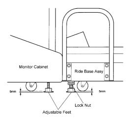
2. Remove 8off security screws (M5x12) and remove both Base Front Cover Plates.
