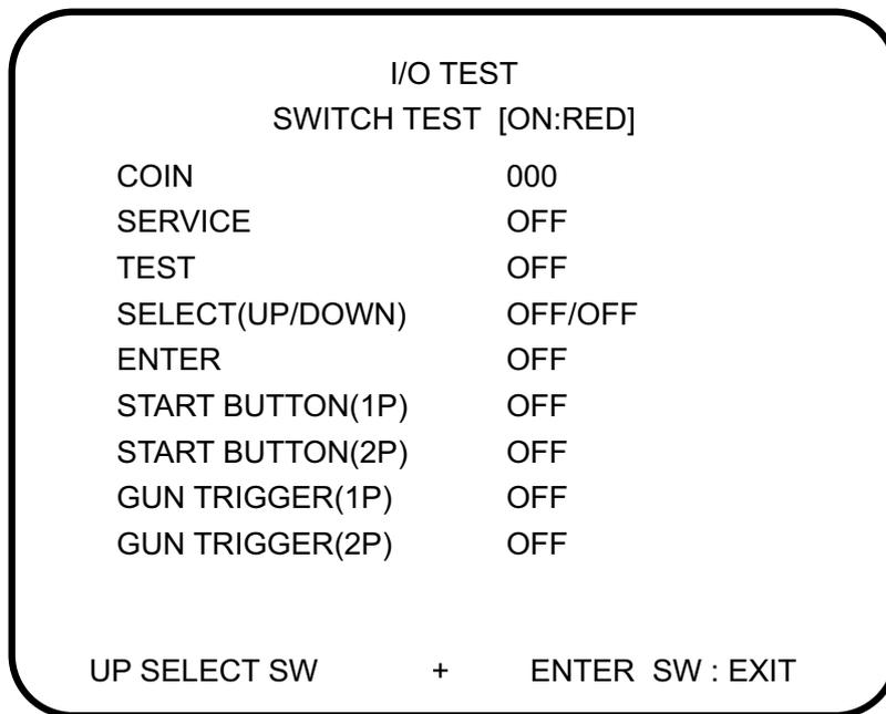
2. The display shows the current state of the switches.
