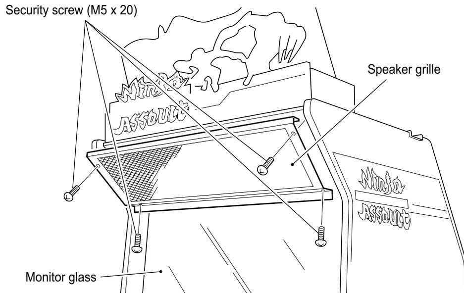
2. Remove 4 off security screw (M5X20) and tilt the Play Panel forwards.
