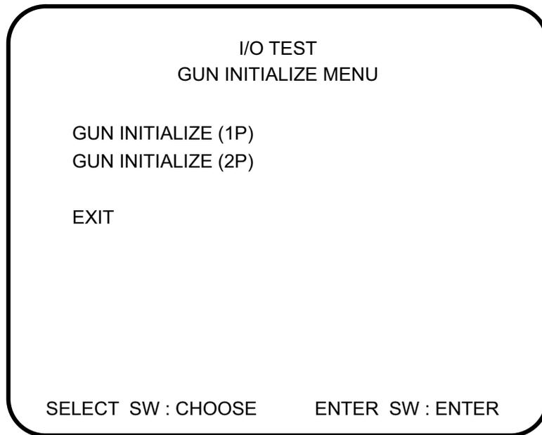
2. Use the Select Up/Down switch to select which gun to Initialize then press the Enter button. The following screen will be displayed.
