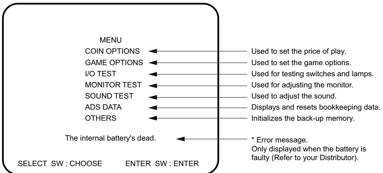
\* Error message (the internal battery is beginning to run down or is faulty.)
