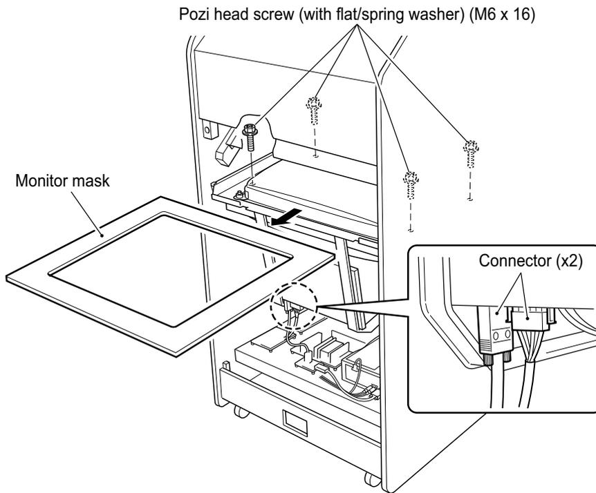
4. Remove the 4 off pozi head screws (M6x16), with flat and spring washers.
