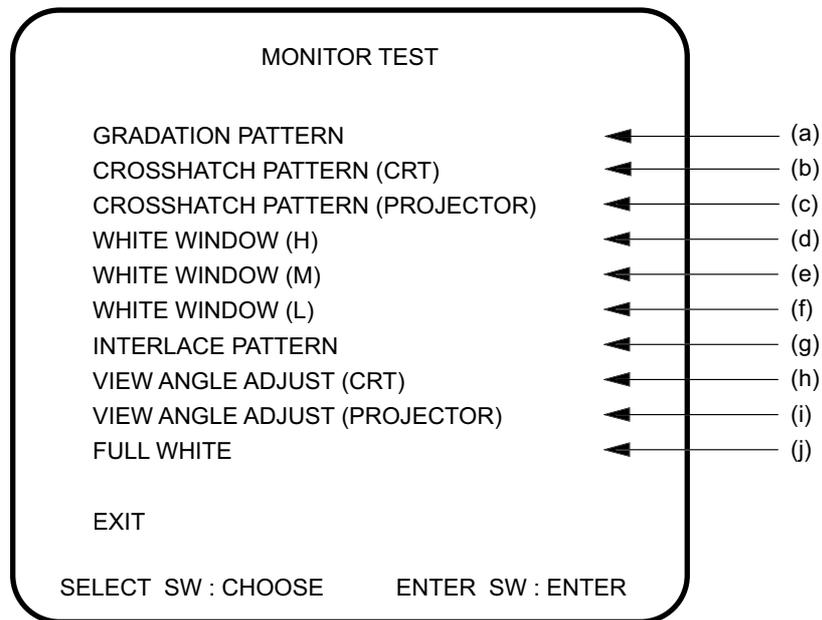
2. Use the Select Up/Down switch to choose the required item then press the Enter button. To return to the Monitor Test Menu from a test pattern press the Enter button.
