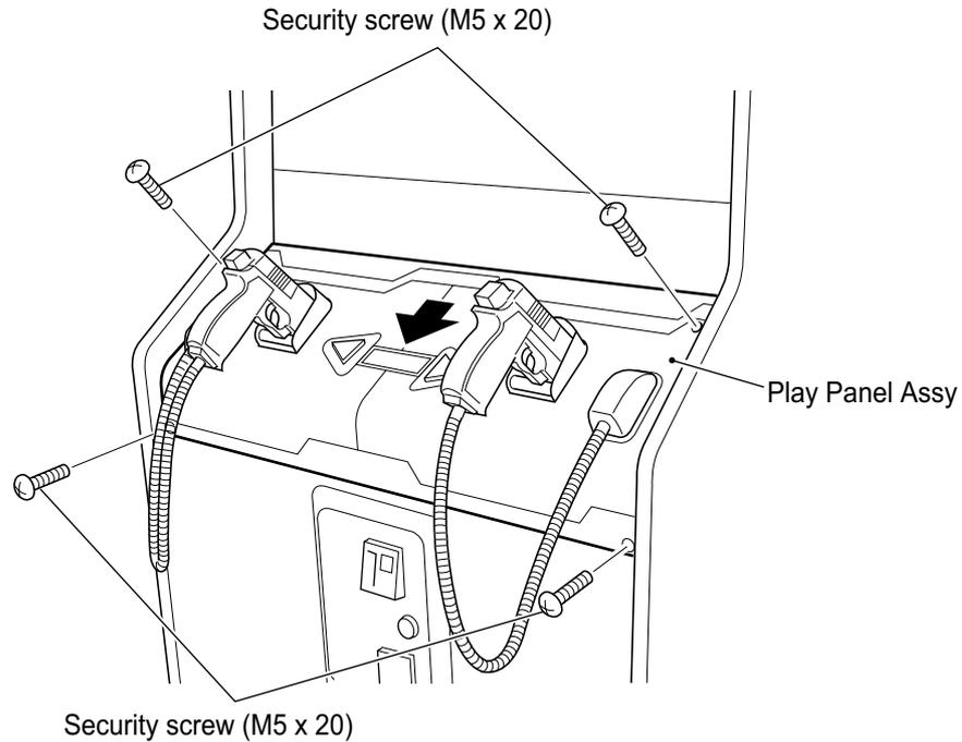
2. Remove the Guns from their holders and allow them to hang down. Tilt the Play Panel forward to gain access to the connectors.
