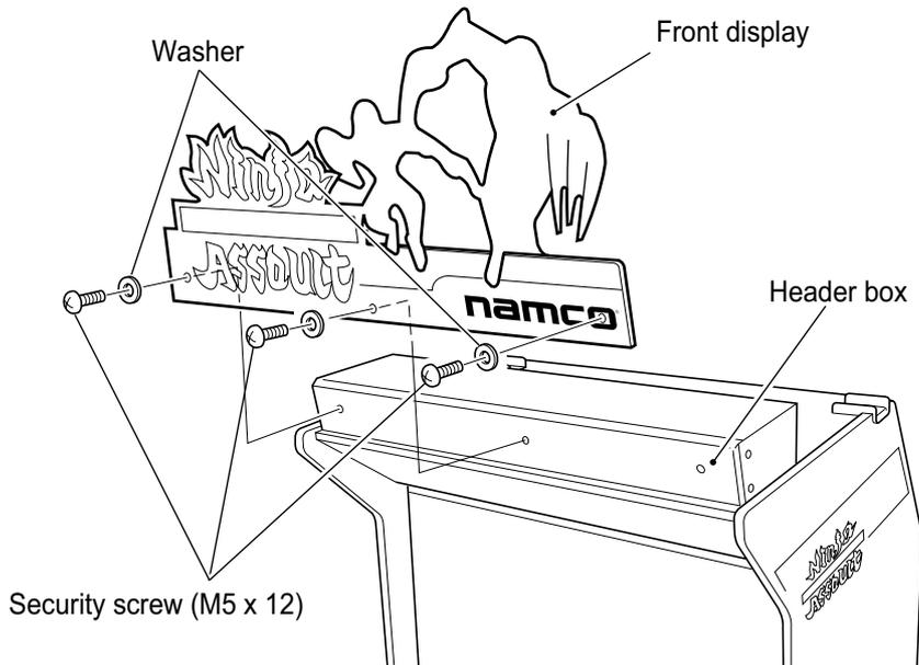
2. Remove 4 off security screw and remove the Front Panel from the Header Box.
