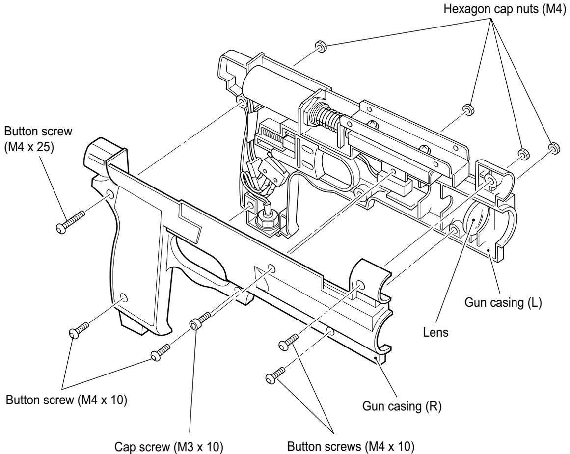
3. Reassemble in reverse order. (Ensure that the flat face of the lens is facing the back of the gun).
