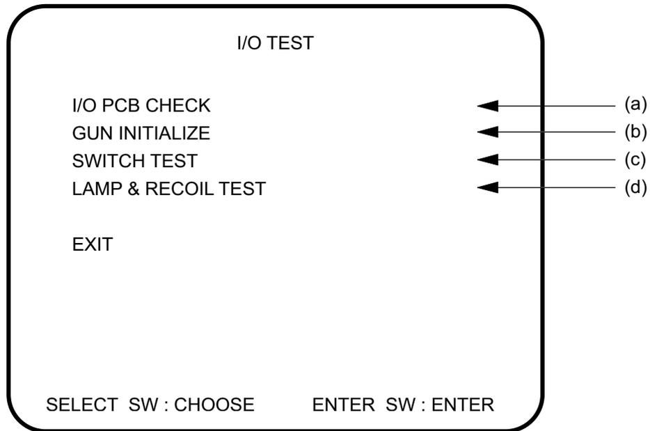
2. Use the Select Up/Down switch to choose the required item then press the Enter button to enter the test.
