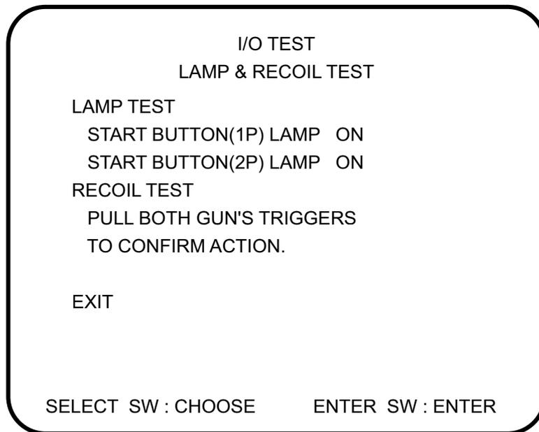
2. Each time a Start Button is pressed the button lamp will turn ON or OFF
