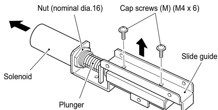
7. Pull out the solenoid plunger, taking care not to lose the spring.
