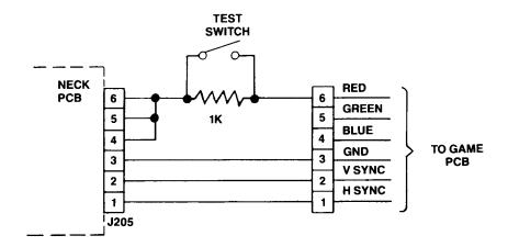
Figure 5-4 Tracking Adjustment Set-Up
