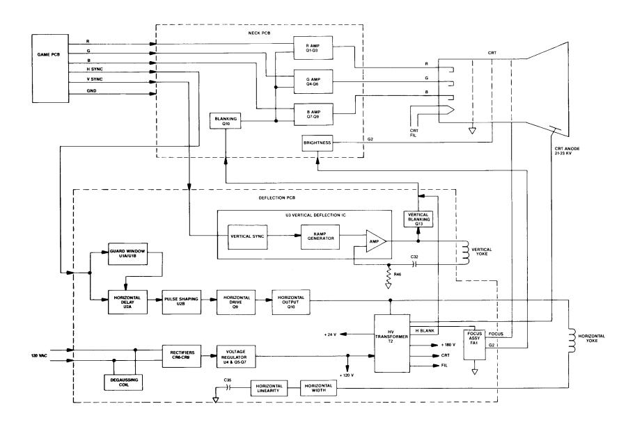
Figure 3-1 Display Block Diagram
