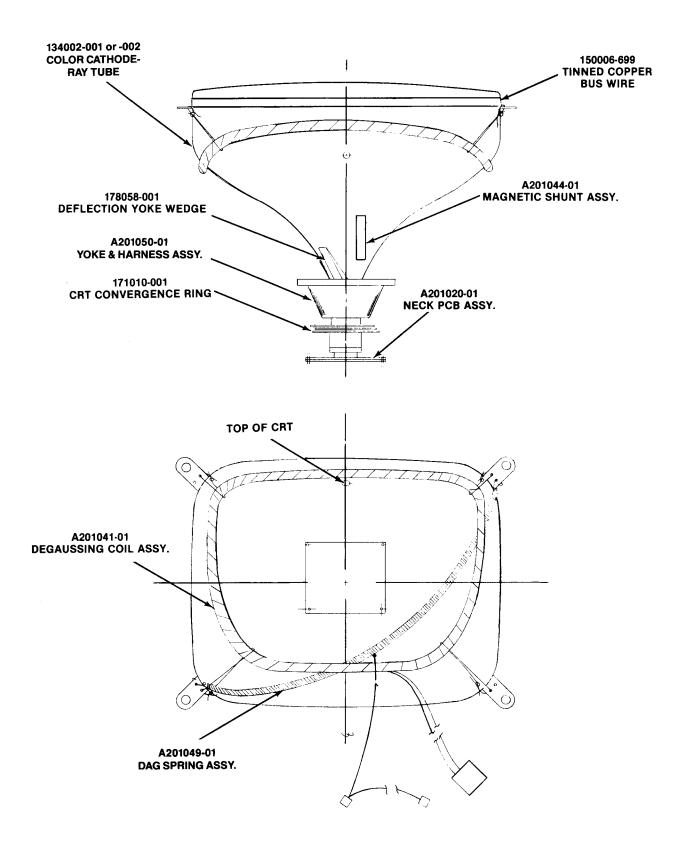
Figure 6-1 Cathode-Ray Tube Assembly 19-Inch Display A201092-01 A
