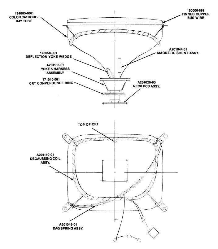
Figure 6-2 Cathode-Ray Tube Assembly 25-Inch Display A201139-01 A
