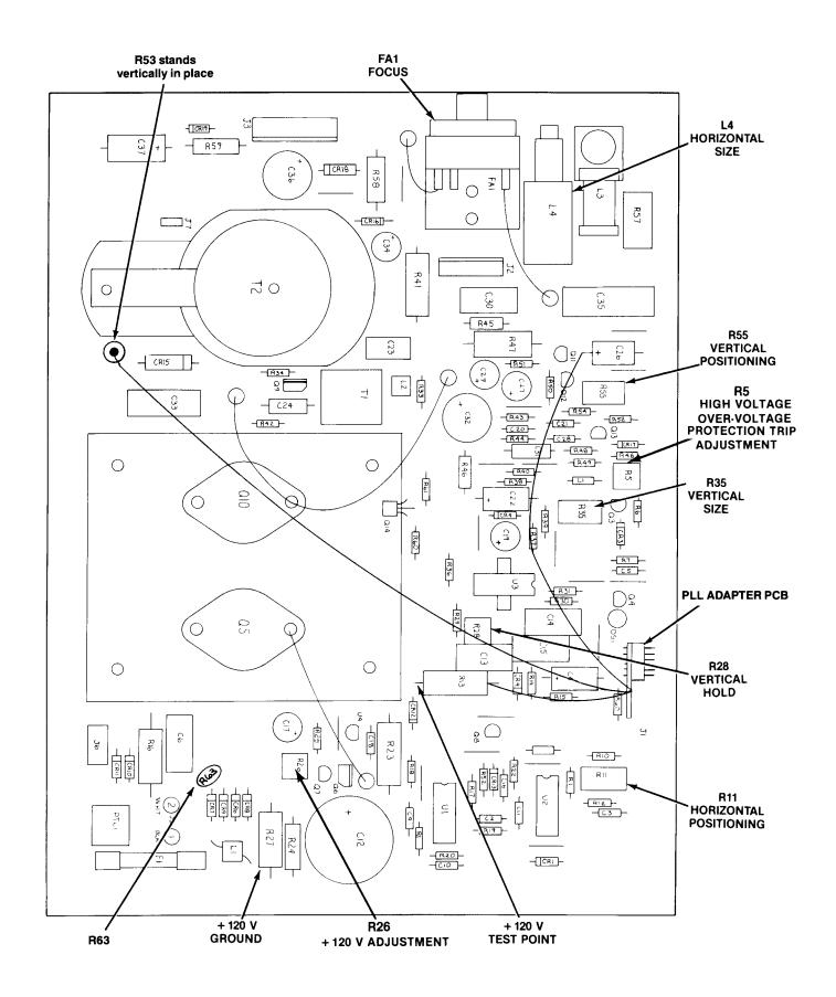
Figure 5-2 Adjustable Controls on the Deflection PCB
