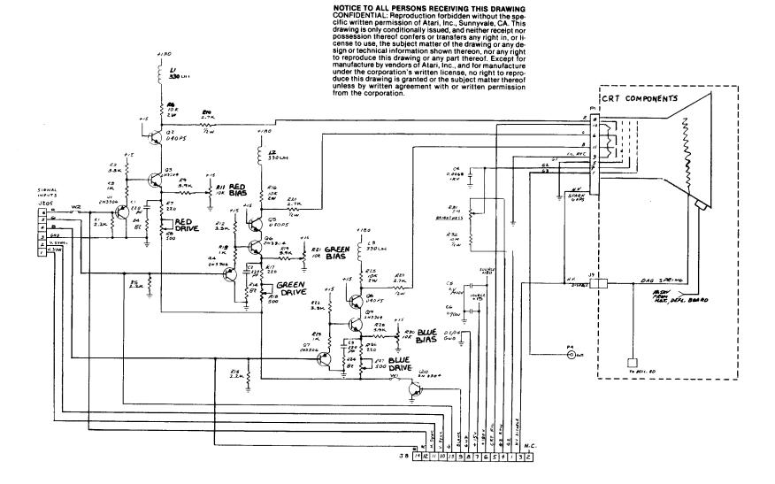
Figure 7-4 Neck PCB Schematic Diagram
