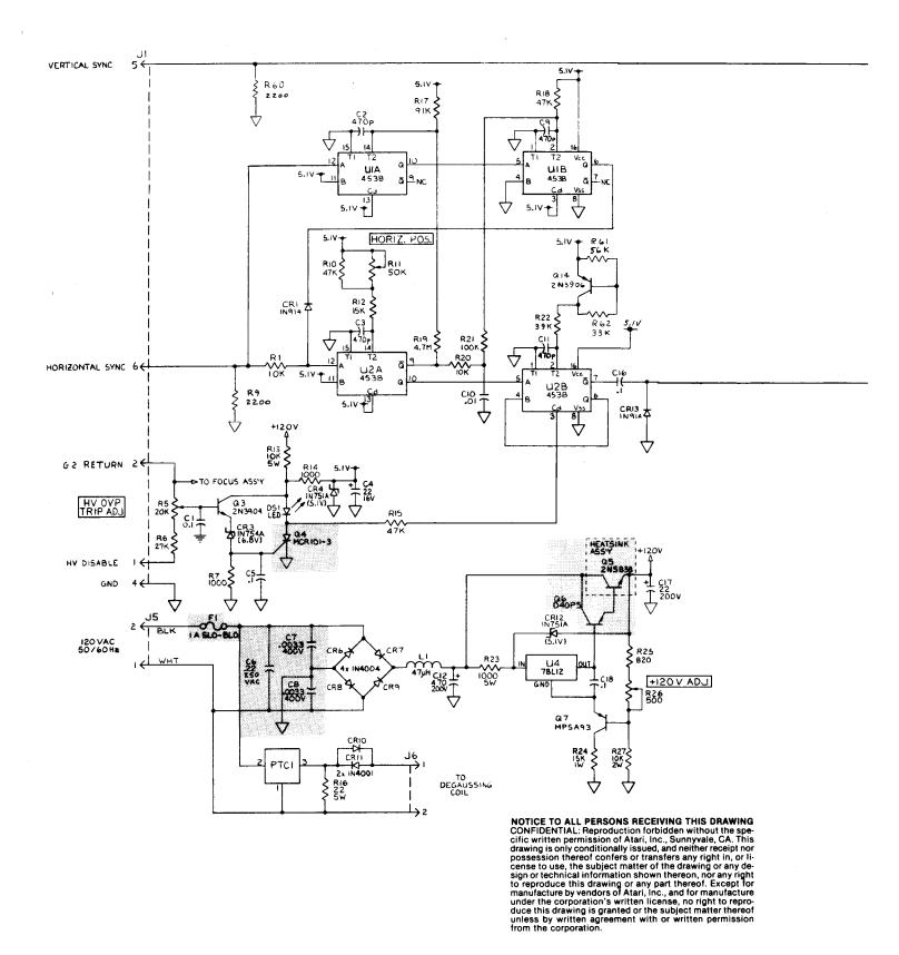
Figure 7-2 19- & 25-Inch Display Deflection PCB Schematic Diagram
