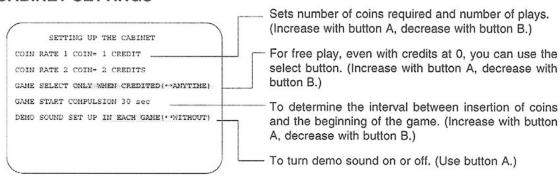
Press button C once to return to soft DIP setting menu. Move the cursor to the desired item and press button A.
