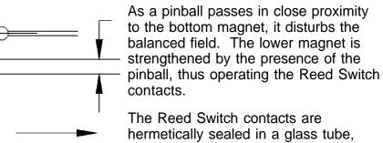
The Reed Switch contacts are hermetically sealed in a glass tube, filled with inert gas to provide long life with stable electrical and operating characteristics. The magnets, the glass tube (with contacts), the Green & White Wires & Diode are sealed in the Plastic Reed Switch Housing in soft epoxy.
