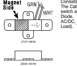
Consists of a Diode (1N4004) and a HSR-042 Reed Switch. The Cable Wiring Harness has the Green Wire going to the switch and the White Wire going to the Anode side of the Diode. The Contact Rating is 100 Volts AC/DC, 0.2 Amps AC/DC, 4 Watts (Resistance Load) & 2 Watts (Inductive Load). The Temperature Operation Range: 0-150° F.
