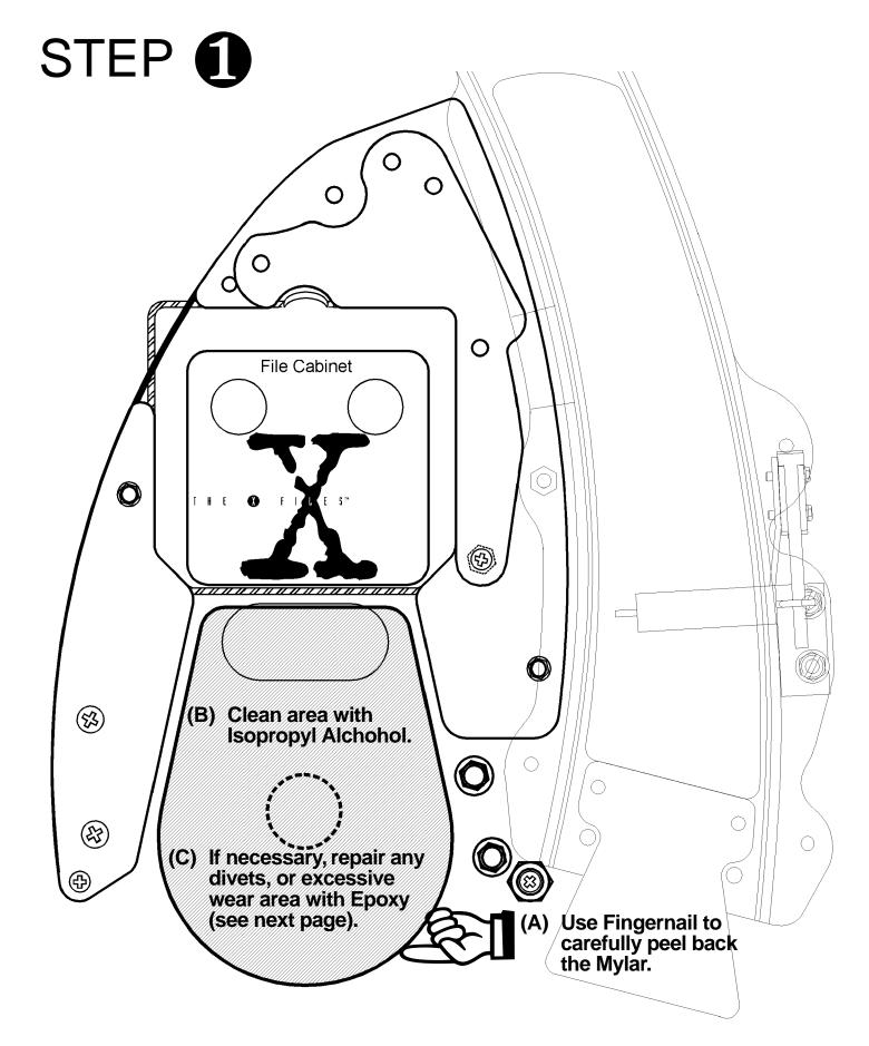
(A) Remove Mylar. (B) Clean Area. (C) If necessary, repair area if diveted or excessive wear.
