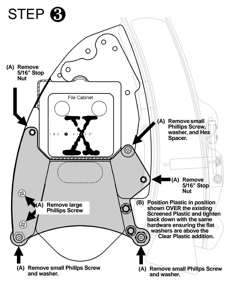
(A) Remove hardware as shown. (B) Position Clear Plastic over area as shown.
