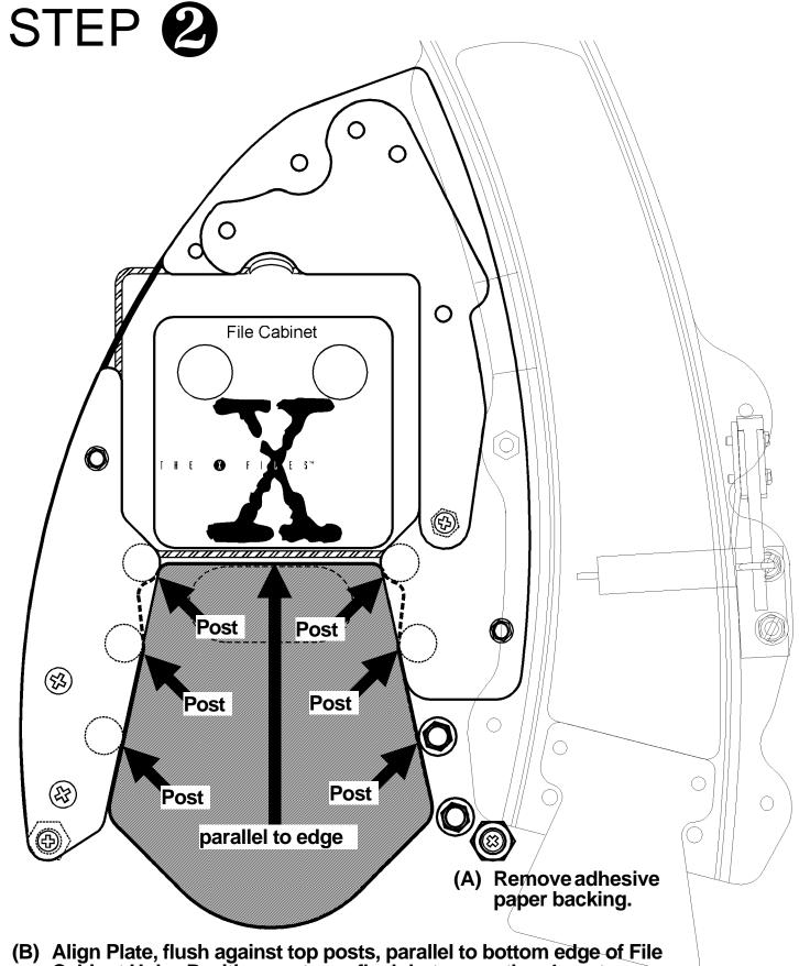
(B) Align Plate, flush against top posts, parallel to bottom edge of File Cabinet Hole. Position center or flush between other 4 posts.
