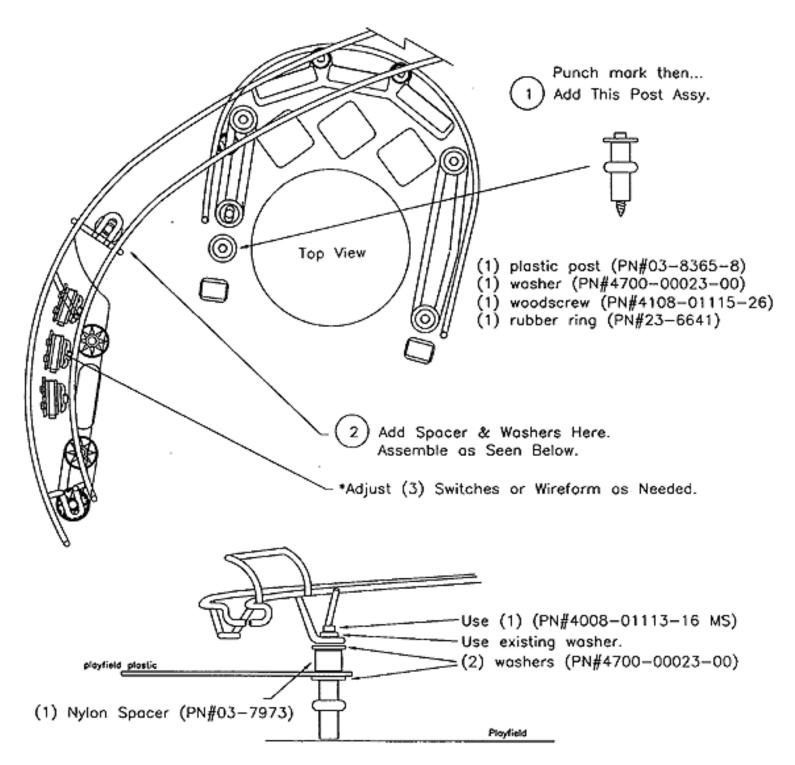
The following is a reduced copy of the template used to punch the hole for the post. A full-sized version is available with the kit or from WMS Parts Service. Use this diagram only as a reference in determining the location of the punch for the post.
