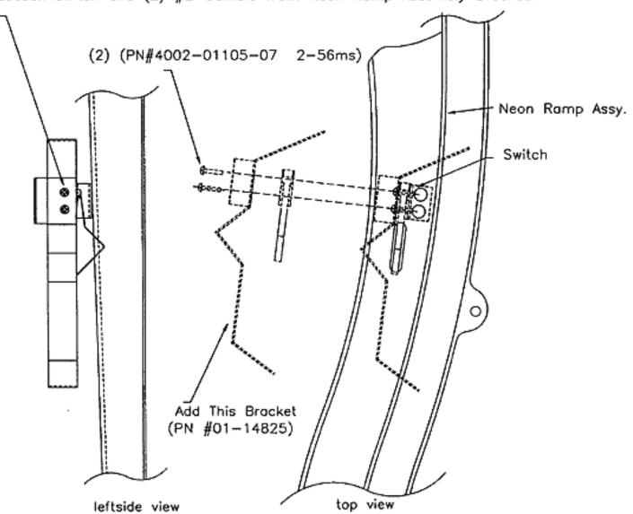
Place Bracket (PN#01-14825) on Switch and re-fasten with the (2) NEW fasteners (PN#4002-01105-07 2-56ms). Tighten gently. The bracket should be to the right of the Spinner Assembly.
